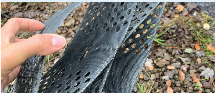
Figure 8. Protecting water quality during all forest management activities is critical. Implementing best management practices, such as installing Geoweb textiles in stream crossings, helps reduce erosion and minimizes soil compaction.
